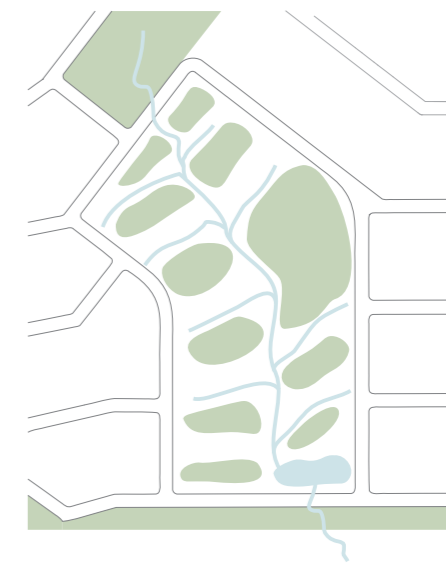
Natural storm water catchment system with new proposed basin system, and newly retained grassland
