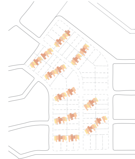
Houses follow the natural terrain, reducing excavation while maximizing view opportunities. Previous allotments are overlaid.
